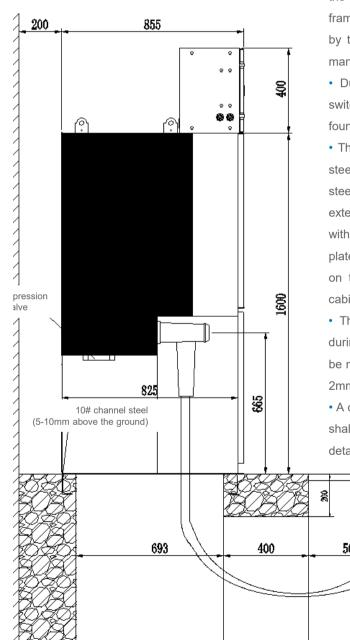
· Generally, the foundation framework shall be buried using secondary pouring method by electrical installation unit after the completion of civil construction, and the foundation framework shall be fabricated based on the drawings prepared by the design department according to the requirements the manufacturer;
